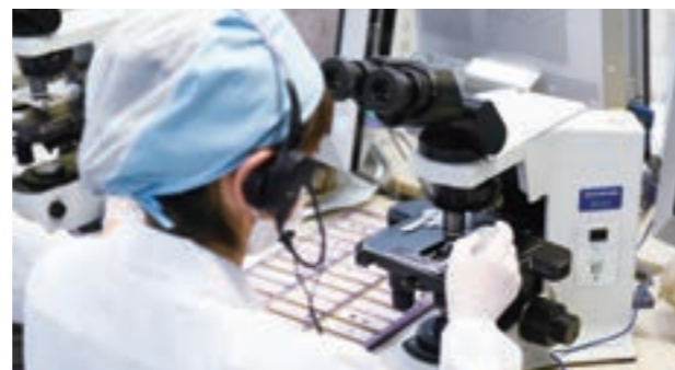
Voice input system to record microscopic examination results
